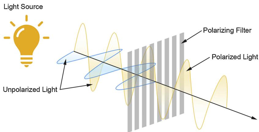
Fig. 1. Schematic diagram of the polarization process.
